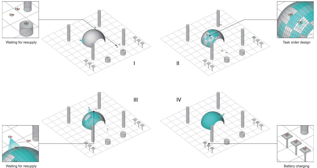
7 Four snapshots of the facade coating simulation, representing another use case scenario of the multi-drone framework.
