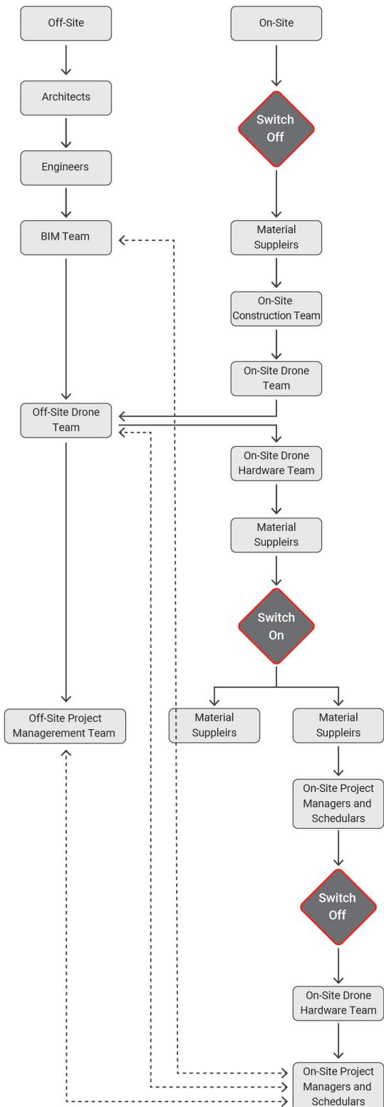
10 Long-term construction workflow pipeline showing different human roles involved and the process for implementing an advanced future framework in an unstructured environment.
